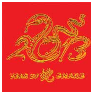
Nanolithography example created by scratching polycarbonate, 20 \mu m scan.
