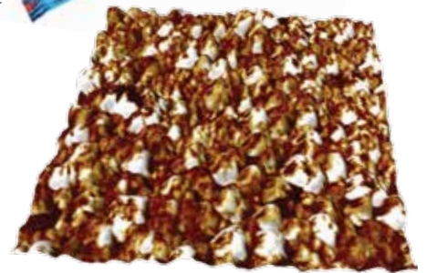
CAFM image of Europium-doped ZnO sample, 2 \mu m scan. Sample courtesy of the Krishnan Lab, Univ. of Washington.
