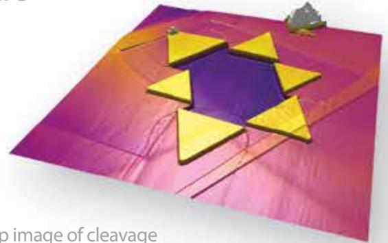
Closed loop image of cleavage defects on graphite surface, 1.7 $\mu$ m scan.
